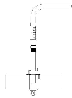
Installation with two (2) FAB-LOK Fastners (FAB-LOK Fasteners Sold Separately)
