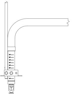
Applications with <sup>3</sup>/<sub>8</sub>" & <sup>1</sup>/<sub>2</sub>" Threaded Rod (Threaded Rod Sold Separately) Institutional - Ceiling or Sidewall
